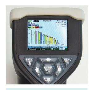
The RIIDEye X operator can view the real-time spectra build of isotopes present in the environment as the identification scan is in process.
