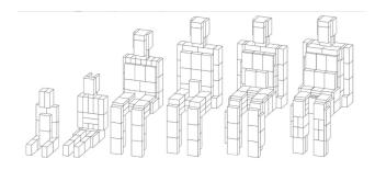
The Whole Body Phantom with radionuclide sources forms a reference sample of activity of incorporated radionuclides uniformly distributed in the human body. This reference sample reproduces the gamma-radiation spatial-energy spectrum of incorporated radionuclides to transfer the activity value of radionuclides to whole body spectrometers by means of its calibration.
