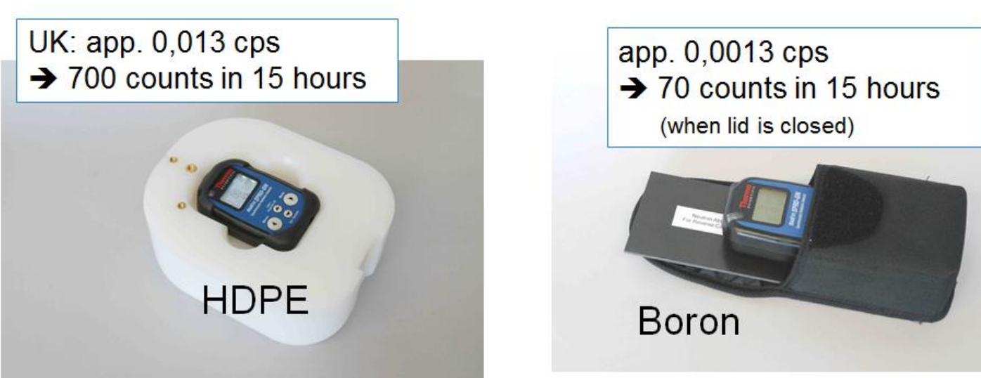
FIGURE 7. Reverse neutron calibration set-up (example)
