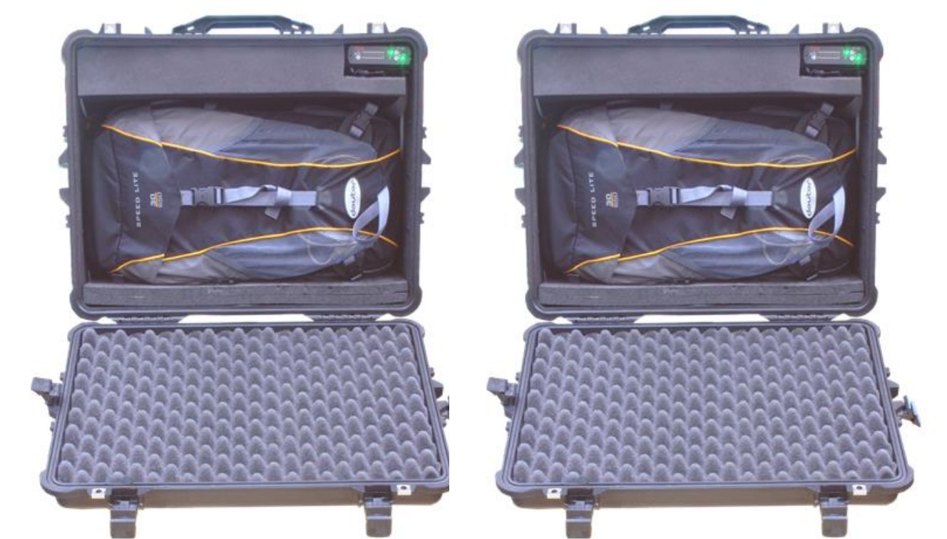
FIGURE 9. Reverse neutron calibration of backpack PackEye FHT 1377 Left: Regular transport and measurement case Right: Special reverse calibration case with inner boron lining
