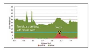
The RadEye PRD provides Advanced NBR with more energy bins to identify even complex mixes of artificial radiation from NORM. And the outstanding detector sensitivity of the RadEye PRD further boosts its NBR performance.
