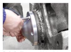
The RadEye GR detector unit is installed quickly and relatively easily at most of the common grapple types. It's compact size takes a minimum of space and so does not significantly impact the grapple's carrying capacity. Check with us for your installation instructions!
