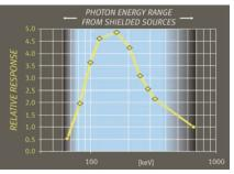
The Thermo Scientific RadEye GR provides superior response to radiation exactly at the energy range of importance to catch shielded radiation sources.
