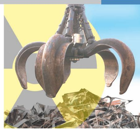
The Thermo Scientific RadEye GR is a radiation detection device designed and proven through extensive testing for the extreme forces and harsh conditions experienced when installed in a grapple. While the detector inside the RadEye GR grapple monitor is smaller than the detectors used in a portal monitor at the entrance of a facility it more than makes up any loss in sensitivity as the RadEye GR detector is much closer (law of 1/r<sup>2</sup> for the
