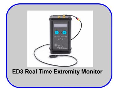
The ED3 Active Extremity Dosemeter allows for simple monitoring of Hp(0.07) for betas and gammas on the extremities with 2 types of probe available depending on the energy.
