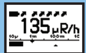
Approaching a source Alarm thresholds - not yet exceeded. Trend arrow indicates increasing radiation level
