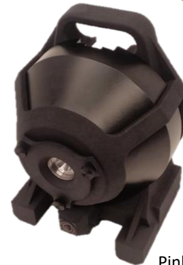
Pinhole Imaging Aperture
