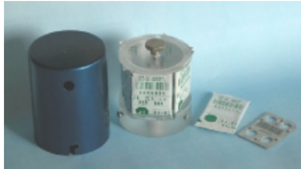
FIG. 1. Photograph of the Seibersdorf H_x area dosimeter. From left to right: aluminium case, PMMA holder for five TLD cards, a packed TLD card, and an unpacked TLD card.
