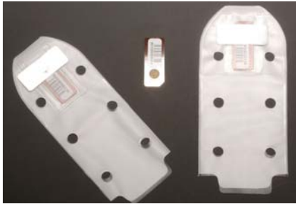
Fig 2. The HPA extremity finger stall dosimeter.
