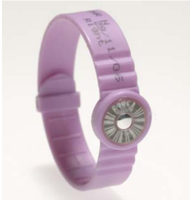
Fig 3. The HPA extremity ring dosimeter.
