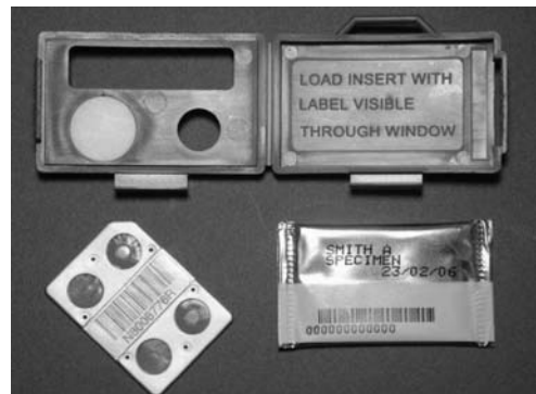
Figure 2. Components of new HPA TLD, including Harshaw TM two-element TLD card using 7 LiF:Mg,Cu,P.
