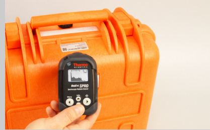
RadEye SPRD for detection/identification of Radionuclides
