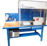
Workstation for melting and casting alloy. Equipped with exhaust system to remove any vapours that might arise during melting of the alloy. The exhaust system is built for performance, yet low noise level (37dB(A) at 3 meters). It offers the ability to control the exhaust volume on control outside the cabinet.
