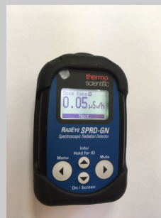
For detection of Gamma & Neutrons
