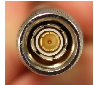
Triax TNC Female (top) and Male (bottom) Part No: Male = PD3
