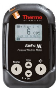
RadEye NL Neutron Survey Monitor is normally worn in a holster. In order to use it as handheld and to increase efficiency, it can be put into an optional moderator with handle #425067110
