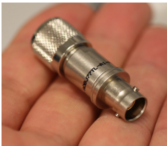
Converter for NPL 2611 Chamber which is now supplied with Triax BNC plug converts to Triax TNC
