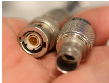
BNC Triax Male (L) and Female (R) Part No: Male = PD1
