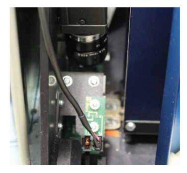
An integrated barcode reader scans cards during processing, time stamping each record, maintaining an unbroken chain of custody and ensuring complete dosimeter data tracking.
